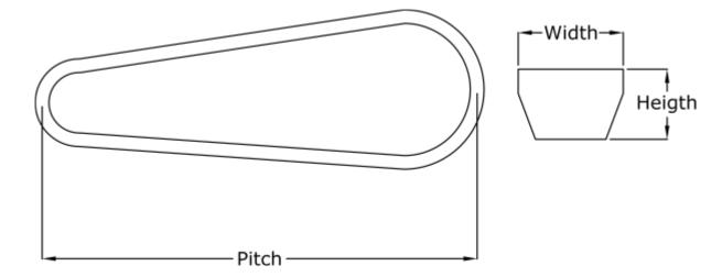
$\begin{array}{ll} \text{Datum Llength} = 5410 \\ \text{Height} &= 10 \\ \text{Length inside} &= 5385 \\ \text{Type} &= \text{BB210} \\ \text{Width} &= 17 \end{array}$
